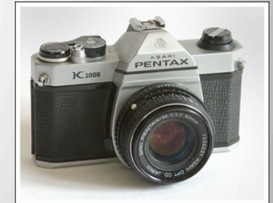
K1000 (Asahi Pentax) Reflex, objectifs interchangeables Film 35mm, format 24x36mm 1976
