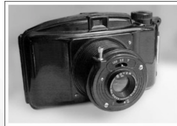
Appareil en bakelite Photax (M.I.O.M.) Film - format 6x9cm – 1946
